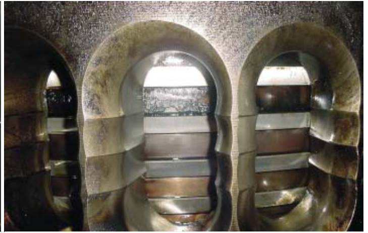
Fig. 6 Typical piston ring condition for a cylinder oil feed rate of 1.0 g/kWh. These are the rings corresponding to Figure 5.
