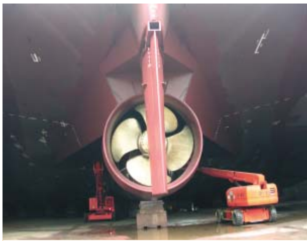
Fig. 10 CPP, HR nozzle and tunnel construction after modification.
