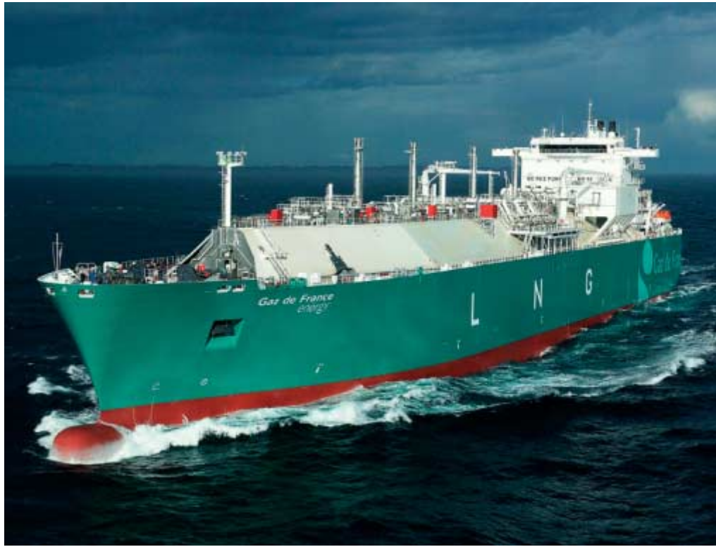
Fig. 1 – The LNG carrier, the 75,000m 3 Gaz de France Energy, is equipped with four 6-cylinder Wärtsilä 50DF engines.
