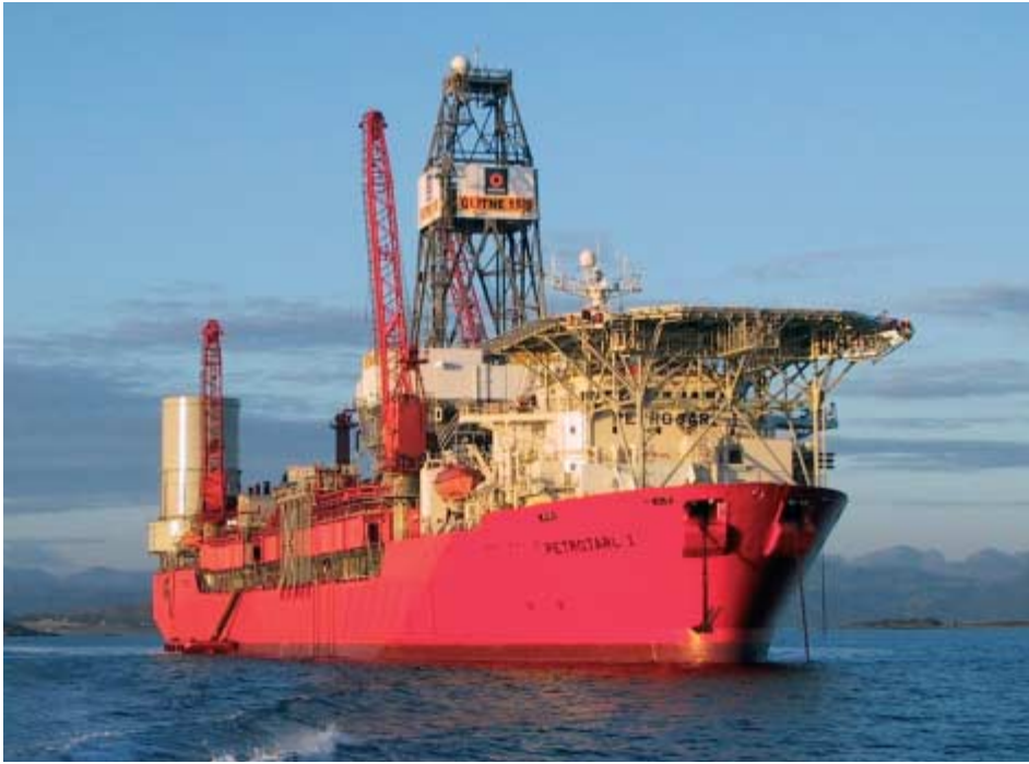
Fig. 3 – Petrojarl 1 with two Wärtsilä 18V32DF prime movers is one of the FPSO's (Floating Production Storage and Offloading vessel) of PGS where Wärtsilä has permanent personnel onboard as a part of the engine room crew.
